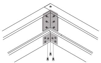
Also fasten the bottom overlap with three tek screws.
