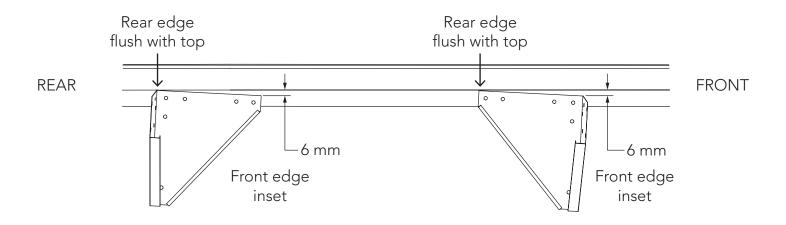
Mark these four hole positions of the BKT07 on the beam and then drill 10 mm holes. Don't fasten these brackets yet, just make the holes for now.
