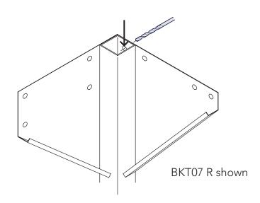
Again using the BKT07 as a template drill these four holes through both sides of the posts and then fasten with four of the longer M10 x 80 mm bolt and a nut with washers both sides.
