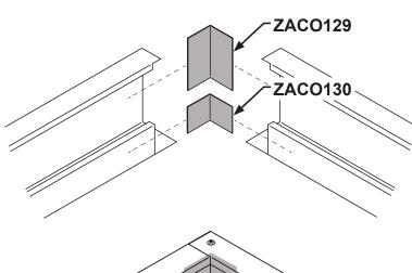
The joiner angles should be positioned on the inside of the edge beams.
