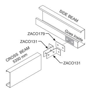
Secure cross beams to the side beams as shown with two M10 x 20 mm bolt and a nut with washers both sides.
